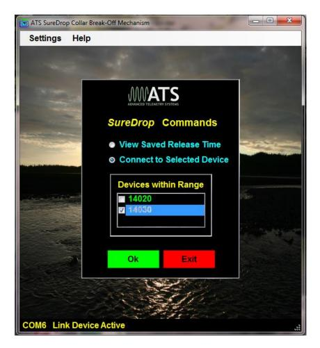
When using the software on the PC for the first time a correct "Com Port" will need to be chosen so the software can communicate with the ATS WS100 Radio Link Dongle. To select the 'Com Port', highlight "Settings" in the toolbar and select "Com Port" from the drop down menu. This will open a dialog box listing the available com ports. Pick your com port and exit.
